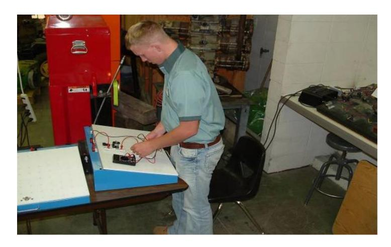
John Deere provides technology services to farmers that include wireless information transfer and satellite guidance systems for equipment operation. Today's John Deere service technicians must be very proficient in electrical/electronic capabilities. At the John Deere Ag Tech Program, I am practicing measuring current flow on a 7810 John Deere tractor circuit. Through this program, I am gaining valuable hands-on experience and mastering skills essential for my internship at Anywhere Equip.
