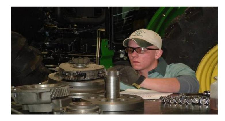
I am disassembling the planetary drive on a John Deere 8420 to check the sun gears for pitting or wear. Ensuring that I am performing the procedure properly, I use a tech manual as a guide. Participating in the John Deere Ag Tech Program, I am learning valuable job skills that are very beneficial in my employment at Anywhere Equipment. Upon completion of the program, I will be awarded an Associate Degree in Applied Science and earned certification with John Deere in electrical/hydraulics
